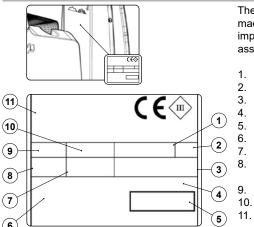
The serial number plate is located at the rear of the steering column, and indicates the machine's general characteristics, including its serial number. The serial number is a very important piece of information and should always be provided together with any request for assistance or when purchasing spare parts. The serial number plate contains the following:
